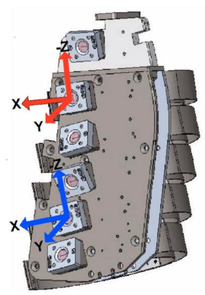
If a SIDIIS or WorldSID RibEye is mounted so that it faces toward the dummy's left side, then the Y data sign must be changed.
